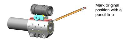
Important: Normal tightening of screws is sufficient. Do not overt-tighten screws. This can lead to a significant loss of the rifle's accuracy.
